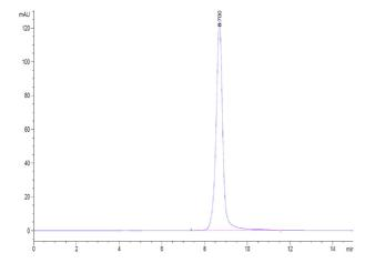
The purity of Biotinylated Human IL-2 R beta is greater than 95% as determined by SEC-HPLC.
