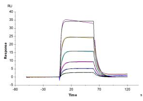
Biotinylated Human IL-2 R beta, His-Avi Tag captured on CM5 Chip via anti-his antibody can bind Human IL-2, No Tag with an affinity constant of 0.079  $\mu$ M as determined in SPR assay (Biacore T200).
